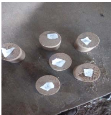
Fig 3: Test Sand Samples For Permeability Test
