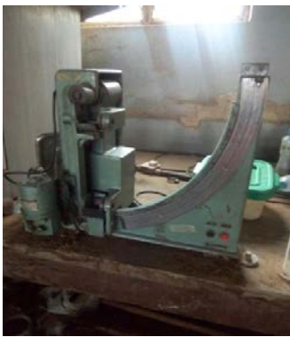
Fig 12: Universal Sand Strength Testing Machine (Ridsadle-Dietert Design, Middles Brough ENG, Serial Number: M8415)
