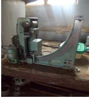
Fig 9: Universal Sand Strength Testing Machine (Ridsadle-Dietert Design, Middlesbrough ENG, Serial Number: M8415)
