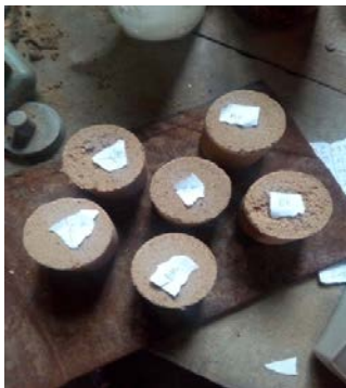
Fig 10: Sand Samples for Green Compression Stress Test
