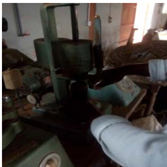
Fig 8: Sand Rammer for Making Sand Test Sample
