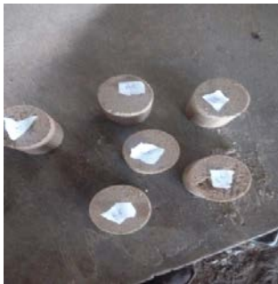
Fig 7: Sand Samples for Dry Compression Stress Test
