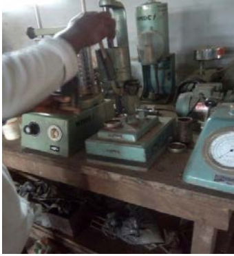
Fig 11: Sand Rammer for Making Sand Test Sample
